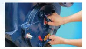
Even during preventive maintenance, internal inspection can be carried out quickly and safely. To do this, all that has to be done is to unscrew and lift the handles of the inspection cover, and then perform the cleaning operation, without removing the casing nor disconnection ten pipework.
