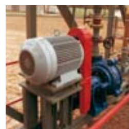
Top: High pressure 20/18 AH slurry pump ready for installation at the Minera Escondida new tailing line.
